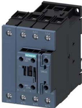
contactor AC-1, 110 A, 400 V / 40 °C, 4-pole, 20-33 V AC/DC, 50/60 Hz, with integrated varistor, auxiliary contacts: 1 NO + 1 NC, screw terminal, size: S2
