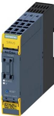
SIRIUS safety relay basic unit 3SK2 series 10 F-DI, 2 F-DQ, 1 DQ, 24 V DC Can be parameterized via SIRIUS Safety ES 22.5 mm overall width spring-loaded terminal (push-in) up to SIL 3 (IEC 62061) up to performance level e (ISO 13849-1) output expansions 3SK1, coupling relay 3RQ1 and fail-safe motor starters 3RM1 via device connector connectable
