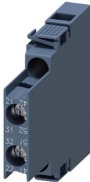
auxiliary switch, lateral, 2 NC, on the left: 41/42, 51/52, on the right: 21/22, 31/32, current path: 1 NC, 1 NC, screw terminal, for contactors 3RT2.1
