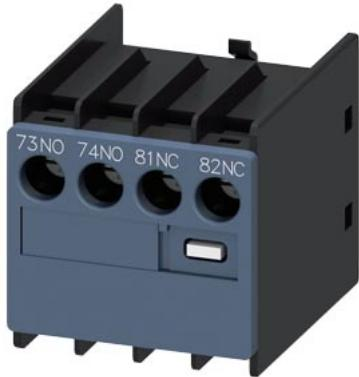
auxiliary switch, on the front, 1 NO + 1 NC, 73/74, 81/82, current path: 1 NO, 1 NC, cable entry from the top, screw terminal, for contactors 3RT2 and contactor relays 3RH2
