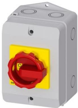
SENTRON, Switch disconnector 3LD, emergency switching-off switch, 3- pole, Iu: 32 A, operating power / at AC-23 A 400 V: 11.5 kW, molded-plastic encapsulation for metric cable gland, rotary operating mechanism, red/yellow
