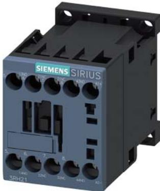
coupling contactor relay, 2 NO + 2 NC, 24 V DC, 0.7-1.25\* Us, with integrated suppressor diode, screw terminal, frame size S00, suitable for PLC outputs, not expandable with auxiliary switch expandable
