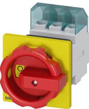
SENTRON, Switch disconnector 3LD, emergency switching-off switch, 3- pole, I<sub>u</sub>: 25 A, operating power / at AC-23 A 400 V: 9.5 kW, front-mounted, rotary operating mechanism, Red / yellow, central mounting 22.5 mm of the handle
