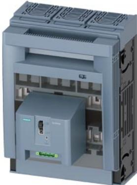
SENTRON, Fuse switch disconnector 3NP1, 3-pole, NH2, 400 A, for assembly and installation on mounting plate, flat terminal, Fuse monitoring: electromechanical, Cover level 70 mm
