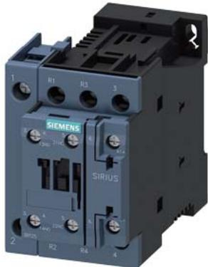
power contactor, AC-3, 25 A, 11 kW / 400 V, 4-pole, 125 V DC, main contacts: 2 NO + 2 NC, auxiliary contacts: 1 NO + 1 NC, screw terminal, size: S0
