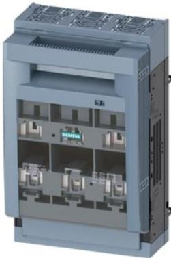
SENTRON, Fuse switch disconnector 3NP1, 3-pole, NH1, 250 A, for Busbar system 8US 60 mm, Box terminal, Cover level 32/70 mm
