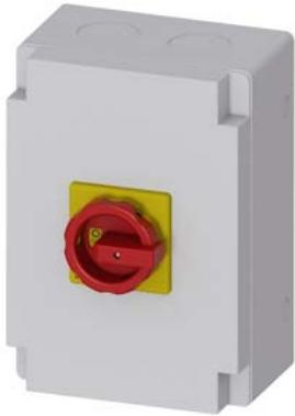
SENTRON, Switch disconnector 3LD, emergency switching-off switch, 3- pole, Iu: 125 A, operating power / at AC-23 A 400 V: 45 kW, Molded plastic encapsulation for metric cable gland, rotary operating mechanism, red/yellow
