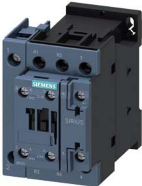
power contactor, AC-3, 25 A, 11 kW / 400 V, 4-pole, 110 V AC, 50 Hz / 120 V, 60 Hz, main contacts: 2 NO + 2 NC, auxiliary contacts: 1 NO + 1 NC, screw terminal, size: S0
