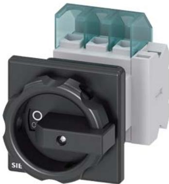
SENTRON, Switch disconnector 3LD, main switch, 3-pole, I<sub>u</sub>: 25 A, Operating power / at AC-23 A at 400 V: 9.5 kW, front-mounted, 1 NC, 1 NO, rotary operating mechanism, black, Central mounting 22.5 mm of the handle
