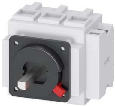
SENTRON, Switch disconnector 3LD, breaker, 3-pole, I<sub>u</sub>: 63 A, Operating power / at AC- 23 A at 400 V: 22 kW, front-mounted, 1 NC, 1 NO, without, Central mounting 22.5 mm of the handle
