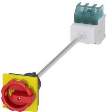
SENTRON, Switch disconnector 3LD, emergency switching-off switch, 3- pole, Iu: 32 A, operating power / at AC-23 A 400 V: 11.5 kW, floor mounting with door coupling, rotary operating mechanism, Red / yellow, 4-hole mounting of the handle
