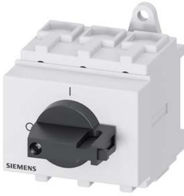
SENTRON, Switch disconnector 3LD, main switch, 3-pole, Iu: 63 A, Operating power / at AC-23 A at 400 V: 22 kW, installation in distribution boards, knob-operated mechanism, black, handle direct at the switch
