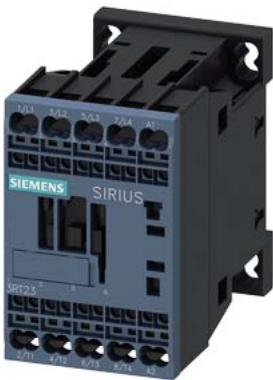
contactor AC-1, 18 A, 400 V / 40 °C, 4-pole, 110 V AC, 50/60 Hz, spring-loaded terminal, size: S00
