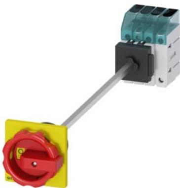
Load disconnector 3LD3, Iu 40 A Main switch 3-pole + N Rated operating capacity at AC-23 A at 400 V 18.5 kW floor mounting Basic switch with door coupling Central hole mounting 22.5mm Rotary actuator red / yellow 66 x 66 mm
