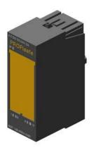
SIPLUS ET 200S F-DQ 24V PROFIsafe based on 6ES7138-4FB04-0AB0 with conformal coating, -25...+60 °C, electronic module for ET 200S, 4 F-DQ PROFIsafe, 24 V DC/2 A, 30 mm overall width, up to category 4 (EN 954-1)/ SIL3 (IEC 61508)/PLE (ISO 13849), can also be used in PROFINET configurations with IM 151-3 HF
