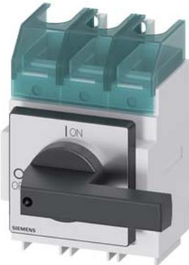
SENTRON, switch disconnector 3LD, main switch, 3-pole,  $I_u$ : 160 A, operating performance / at AC-23 A at 400 V: 75 kW, installation in distribution boards, knob-operated mechanism, black, handle direct at the switch
