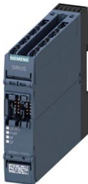
SIRIUS, interface module PROFINET interface for safety relay 3SK2 from E05 and 3RK312/3RK313 from E04 PROFINET IO interface 100 Mbps, RJ45 22.5 mm width screw terminal parameter assignment via Safety ES without connection cable
