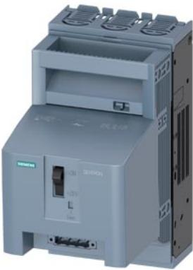
SENTRON, Fuse switch disconnector 3NP1, 3-pole, NH00, 160 A, for assembly and installation on mounting plate, flat terminal, Fuse monitoring: electromechanical, Cover level 45 mm
