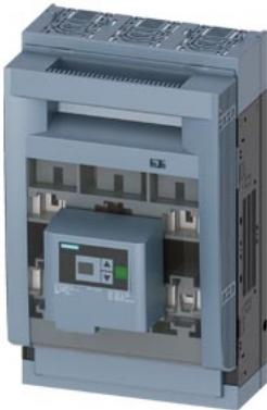
SENTRON, Fuse switch disconnector 3NP1, 3-pole, NH1, 250 A, for assembly and installation on mounting plate, Box terminal, Fuse monitoring: electronic EFM20, Cover level 70 mm
