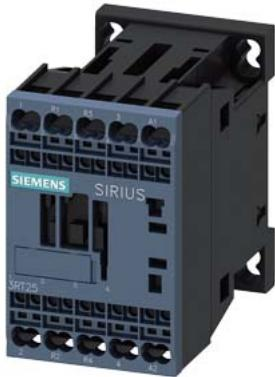
power contactor, AC-3, 12 A, 5.5 kW / 400 V, 4-pole, 230 V AC, 50/60 Hz, main contacts: 2 NO + 2 NC, spring-loaded terminal, size: S00
