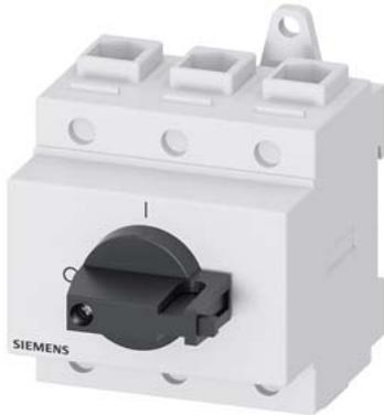
SENTRON, Switch disconnecter 3LD, main switch, 3-pole, Iu: 100 A, Operating power / at AC-23 A at 400 V: 37 kW, installation in distribution boards, knob-operated mechanism, black, handle direct at the switch
