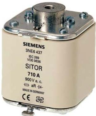
SITOR fuse link, with female thread on both sides, In: 710 A, gR, Un AC: 900 V, front indicator
