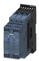
SIRIUS soft starter S2 45 A, 30 kW/500 V, 40  $^{\circ}\text{C}$  400-600 V AC, 24 V AC/DC Screw terminals Thermistor motor protection
