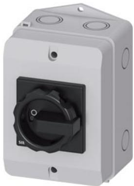
SENTRON, Switch disconnector 3LD, main switch, 3-pole, I<sub>u</sub>: 32 A, Operating power / at AC-23 A at 400 V: 11.5 kW, molded-plastic encapsulation for metric cable gland, rotary operating mechanism, black
