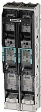
Fuse switch disconnector 3-pole selectable, for protection of transformers on the secondary side up to 1000 kVA for LV HRC fuses GTR 2x722 A max., 400 V AC, and NH3 disconnecting blade up to 2000 A
