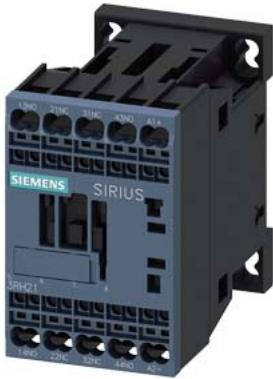
contactor relay, 2 NO + 2 NC, 125 V DC, spring-loaded terminal, frame size S00
