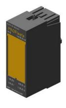
SIPLUS ET 200S EM F-DI 24V PROFIsafe based on 6ES7138-4FA05-0AB0 with conformal coating, -25...+60 °C, electronic module for ET 200S, 4/8 F-DI PROFIsafe, 24 V DC, 30 mm overall width, up to category 4 (EN 954-1)/ SIL3 (IEC 61508)/PLE (ISO 13849), can also be used in PROFINET configuration with IM 151-3 HF
