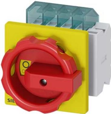
SENTRON, Switch disconnector 3LD, emergency switching-off switch, 4- pole, Iu: 16 A, operating power / at AC-23 A 400 V: 7.5 kW, front-mounted, 1 NC, 1 NO, rotary operating mechanism, Red / yellow, 4-hole mounting of the handle
