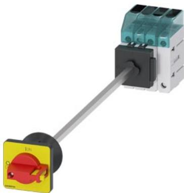
Load disconnector 3LD3, Iu 63 A Main switch 3-pole + N Rated operating capacity at AC-23 A at 400V 22.0 kW floor mounting Basic switch with door coupling Central hole mounting 22.5mm Toggle drive red / yellow 48x48 mm
