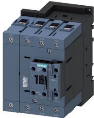
contactor AC-1, 110 A, 400 V / 40 °C, 4-pole, 220 V AC, 50/60 Hz, auxiliary contacts: 1 NO + 1 NC, screw terminal, size: S3
