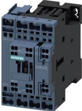
contactor AC-1, 50 A, 400 V / 40 °C, 4-pole, 24 V DC, auxiliary contacts: 1 NO + 1 NC, spring-loaded terminal, size: S0
