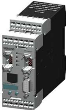
SIRIUS, interface module DP interface, for modular safety system 3RK3 PROFIBUS DP interface 12 Mbps, RS 485 45 mm overall width spring-type terminal can be parameterized via Safety ES without connection cable
