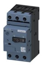
Circuit breaker size S00 for motor protection, CLASS 10 A-release 3.5...5 A N release 65 A Screw terminal Standard switching capacity
