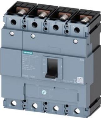
circuit breaker 3VM1 IEC frame 250 breaking capacity class M Icu=55kA @ 415V 4-pole, line protection TM220, ATFM, In=200A overload protection Ir=140A...200A short-circuit protection li=10 x In N conductor protection 100% nut keeper kit
