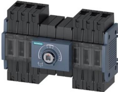
SENTRON, 3KC transfer switching equipment, manually operated, MTSE, size: 1, 3-pole,  $I_{\text{u}}$ : 63 A,  $U_{\text{e}}$  AC: 415 V,  $I_{\text{e}}$  at AC-33 B at 415 V: 63 A,  $I_{\text{e}}$  at AC-23 A at 690 V: 63 A, screw and standard mounting rail installation 35 mm, Front operating mechanism, centered, without handle, box terminal
