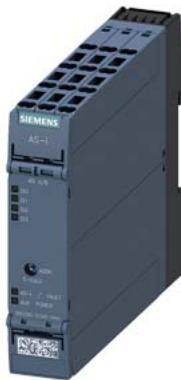
AS-i SlimLine Compact module SC22.5 digital, A/B slave 4 DI, IP20 4 x inputs for 3-wire sensor Sensor supply can be switched over spring-type terminals Overall width 22.5 mm
