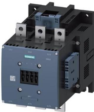
power contactor, AC-3e/AC-3 500 A, 250 kW / 400 V AC (50-60 Hz) / DC Uc: 200-277 V PLC input 24 V DC 3-pole, auxiliary contacts 2 NO + 2 NC drive: electronic main circuit: busbar control and auxiliary circuit: spring-loaded terminal
