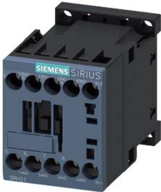
coupling contactor relay, 4 NO, 24 V DC, 0.7-1.25\* Us, with integrated suppressor diode, screw terminal, frame size S00, suitable for PLC outputs, not expandable with auxiliary switch expandable
