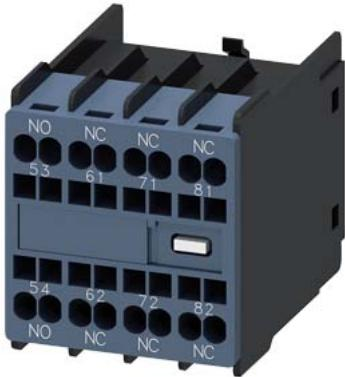
auxiliary switch, on the front, 1 NO + 3 NC, 53/54, 61/62, 71/72, 81/82, current path: 1 NO, 1 NC, 1 NC, 1 NC, spring-loaded terminal, physically coded, only with contactor relays 3RH2140 and 3RH2440 combinable (according to EN 50011)
