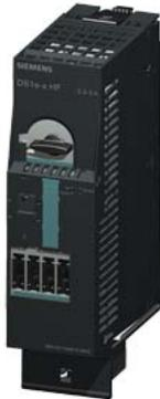
DS1E-X for ET200S High Feature DOL starter Setting range 0.3...3 A Mechanical switching Electronic protection AC-3, up to 1.1 kW / 400 V expandable for brake control module 2DI module Motor starter ES Circuit breaker signaling parameterizable DPV 1-capable PROFIENERGY-capable to PN
