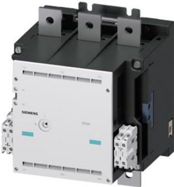
vacuum contactor AC-3e 630 A, 335 kW / 400 V, AC-3 820 A, 450 kW / 400 V, Ue 1000 V, 3-pole, Uc: 200-240 V AC(50/60 Hz) drive: conventional auxiliary contacts 4 NO + 4 NC main circuit: busbar control and auxiliary circuit: screw terminal
