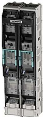
Fuse switch disconnector 3-pole selectable, for protection of transformers on the secondary side up to 500 kVA for LV HRC fuses GTR 722 A max., 400 V AC, and NH3 Disconnecting blade up to 1000 A
