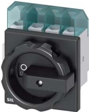
SENTRON, Switch disconnector 3LD, main switch, 4-pole,  $I_{u}$ : 25 A, Operating power / at AC-23 A at 400 V: 9.5 kW, front-mounted, rotary operating mechanism, black, 4-hole mounting of the handle
