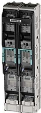
Fuse switch disconnector 3-pole selectable, for protection of transformers on the secondary side up to 800 kVA for LV HRC fuses GTR 2x577 A max., 400 V AC, and NH3 disconnecting blade up to 1600 A
