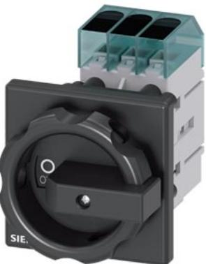
Load disconnector 3LD3, Iu 40 A Main switch 3-pole Rated operating capacity at AC-23 A at 400 V 18.5 kW Front plate mounting Basic switch with Central hole mounting 22.5mm Toggle drive black 66x66 mm
