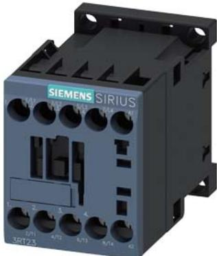
contactor AC-1, 22 A, 400 V / 40 °C, 4-pole, 230 V AC, 50/60 Hz, screw terminal, size: S00
